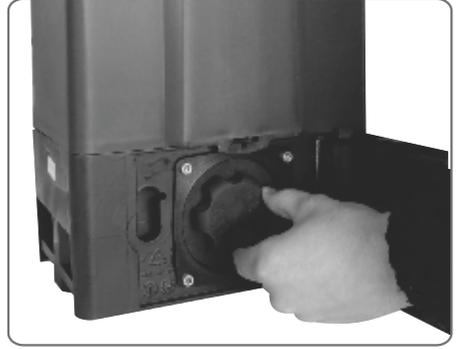
2. Ensure that the gearbox is engaged by turning the thumbwheel anti-clockwise before fitting the **Thumbwheel Guard**. It must not be possible to move the gate by hand.
